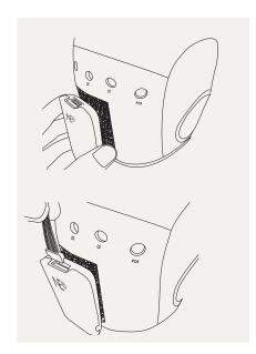
The Necbox is attached to the neoprene cap using the velcro, and it is connected to the electrode cable using the 10-pin connector.
